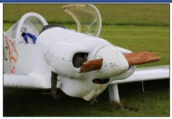
Photo No. 4: Damage to EI-EWZ
