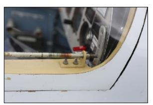
Photos No. 2 and 3: Detail of Canopy Locking Mechanism
